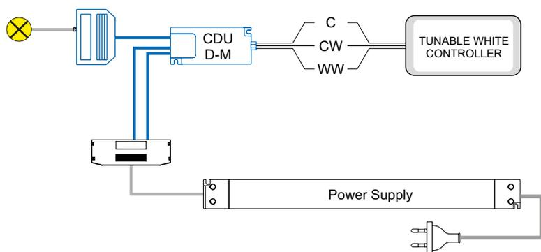
Example of parallel connection with a single power supply. Digital control systems (Switch Controllers) are not supplied by Domus Line. Only connect Domus Line luminaires with dual-colour D-M light sources.
