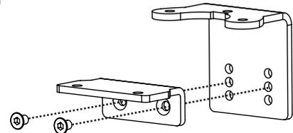
If required change the clamp plate setting by removing Countersunk screws and adjusting to correct setting
