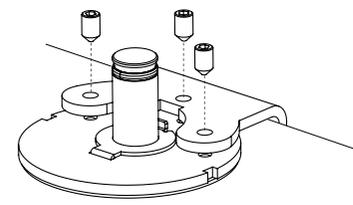
**6 TIGHTEN GRUB SCREWS INTO POSITION**
