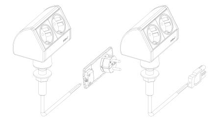
Fixed Power Supply Cable routed through the stainless steel pillar.
