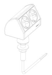
Fixed Power Supply Cable routed through the stainless steel pillar.
