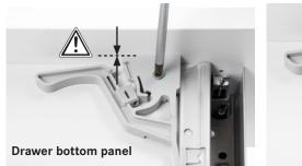
Position child lock flush with the front panel and, screw to the drawer bottom panel using a  $4 \times 20$  mm countersunk screw.
