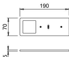
**POLAR SE** is a luminaire made entirely of aluminium with a thickness of only 5mm. The luminaire integrates a special **LGP LED** cluster which offers a wide and diffused light projection, without the dot-effect. **POLAR SE** has been designed for rapid mounting on the surface and on the wall with only two screws. This makes it possible to conceal the power cable directly on the back of the cabinet without having to plan preventive and complex holes in the cabinet.
